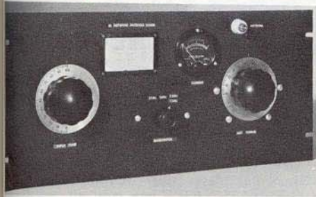
PANEL VIEW of the one-kilowatt pi-network antenna tuner at W2FBS, constructed on an 8 3/4 x 19-inch aluminum relay rack panel. National type "O" dials are on C 1 and C 2 .
