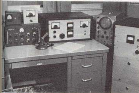
MONITOR-ADAPTED 'SCOPE AT K21OW, at right of desk, a Heath type O-5 constructed from a kit. Space for the adapter components and additional panel controls can be found in most test type oscilloscopes.
